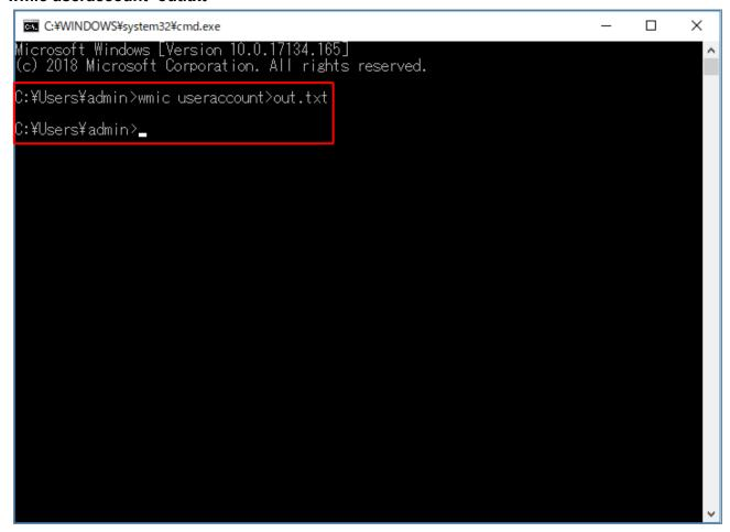
[2] Open the "out.txt" generated in the Command Prompt's current directory with a text editor. Copy the "SID" for the user to set up web filters for.
